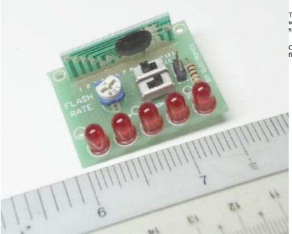
This cmos VLSI single chip-on-board is designed for electronic toy and warning light applications. Five LED's flash on/off in a pseudo-random or sequential mode depending on whether a switch is open or connected high.
